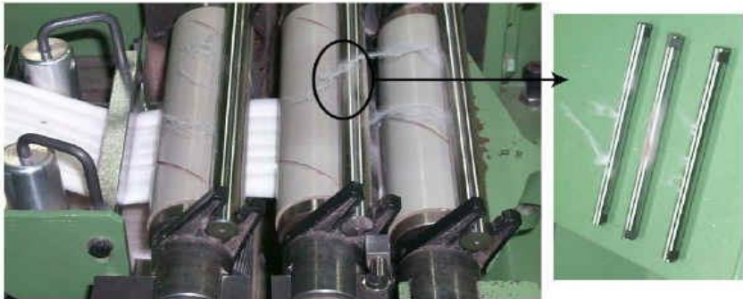
Fig. 3. Sticky deposits on the drafting section of the draw frame.
