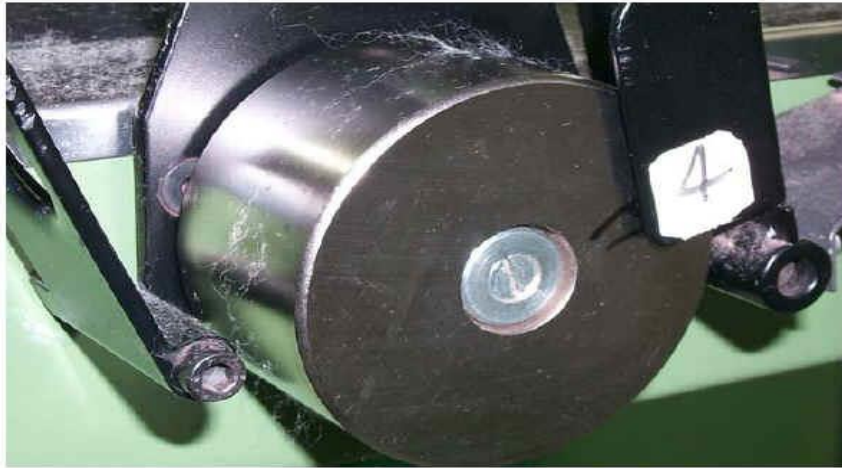
Fig. 2. Sticky deposits on the draw frame creel drive rolls.
